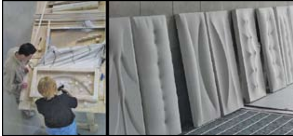
Figure 1: Model formwork and completed plaster casts. Courtesy of C.A.S.T.
