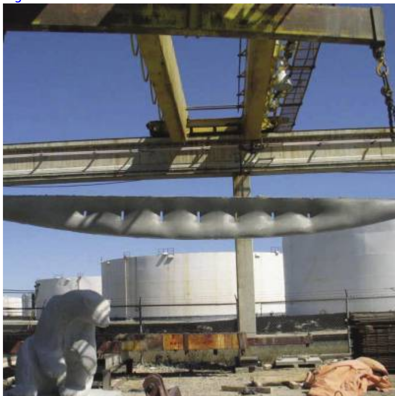
Fig. 8. Completed full scale variable section concrete 'pinch' beam.
