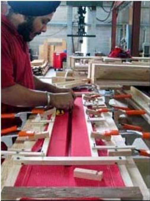
Fig. 1. Model beam formwork.
