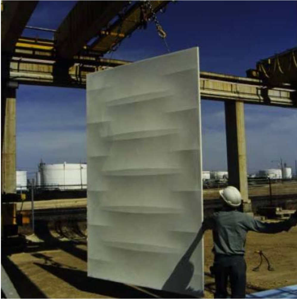
Fig. 11. Completed full scale reverse cast GFRP panel.
