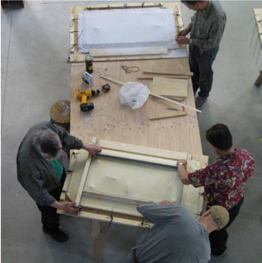
Fig. 2. Model wall panel formwork.
