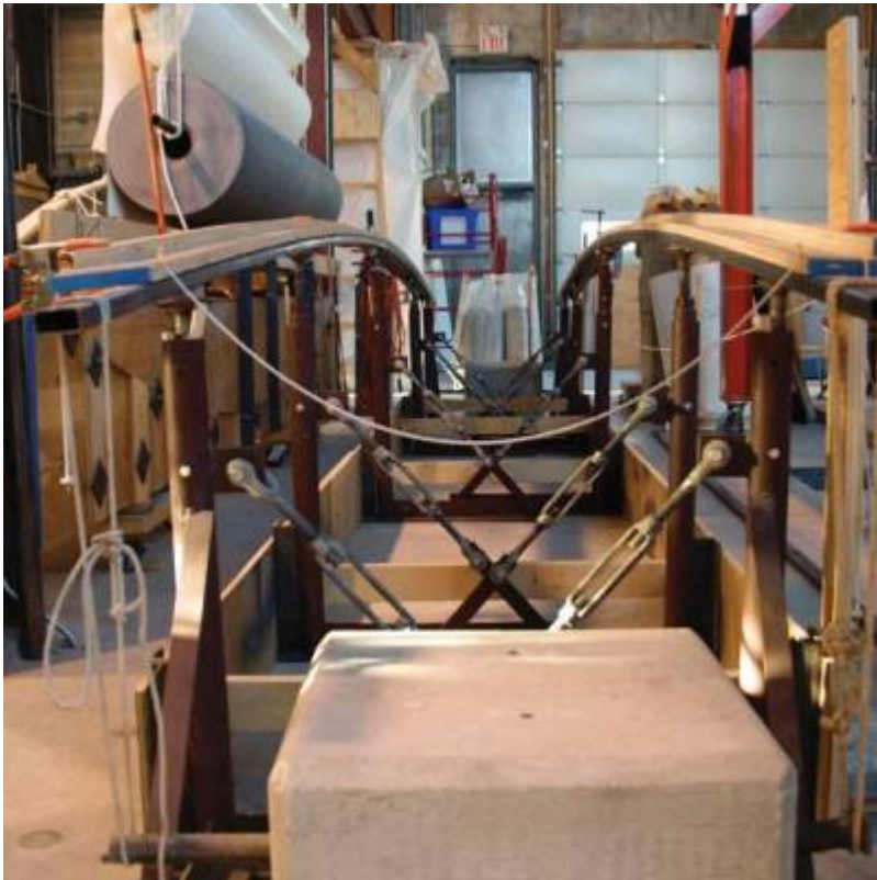
Fig. 32. Simple perimeter frame used to support fabric mold to form double...
