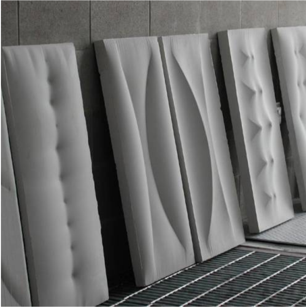
Fig. 3. Completed wall panel plaster casts.
