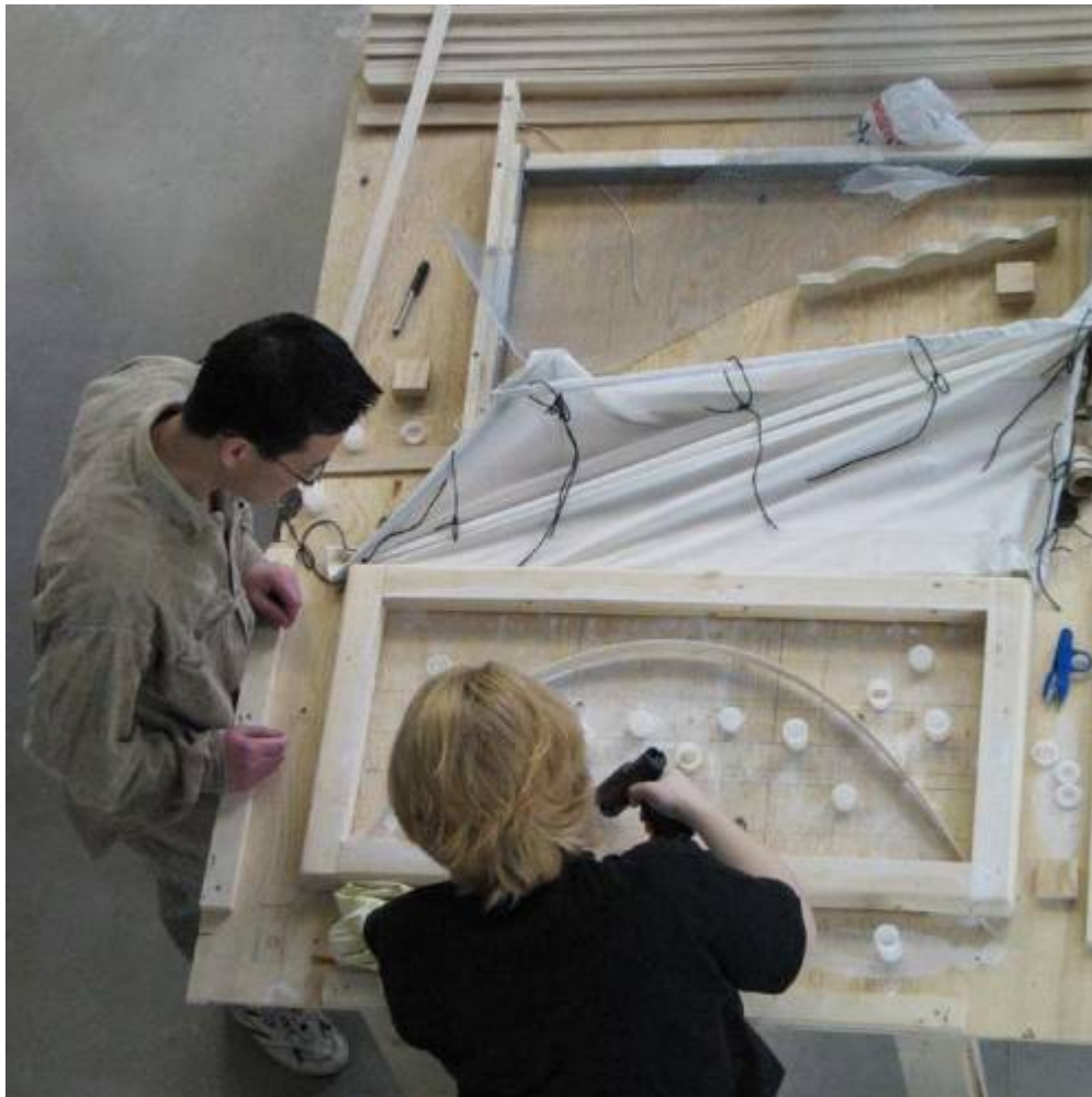
Fig. 1. Model wall panel formwork.
