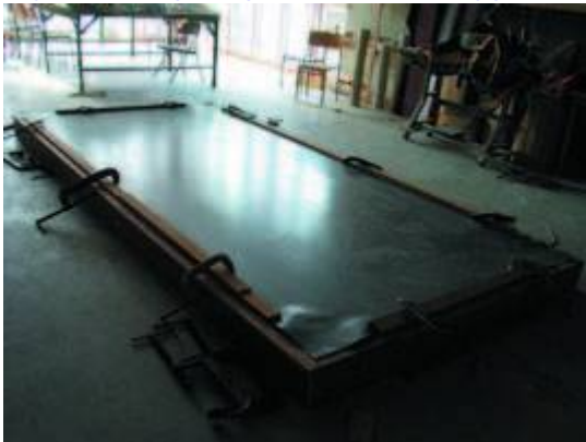
Fig. 27. Coated woven polyethylene fabric is stretched and secured to the open...
