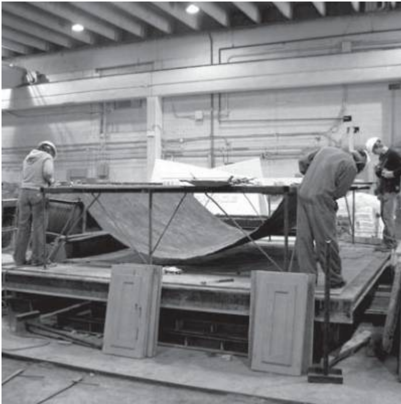
Fig. 22. Step 1 - Geotextile fabric hung from a frame.
