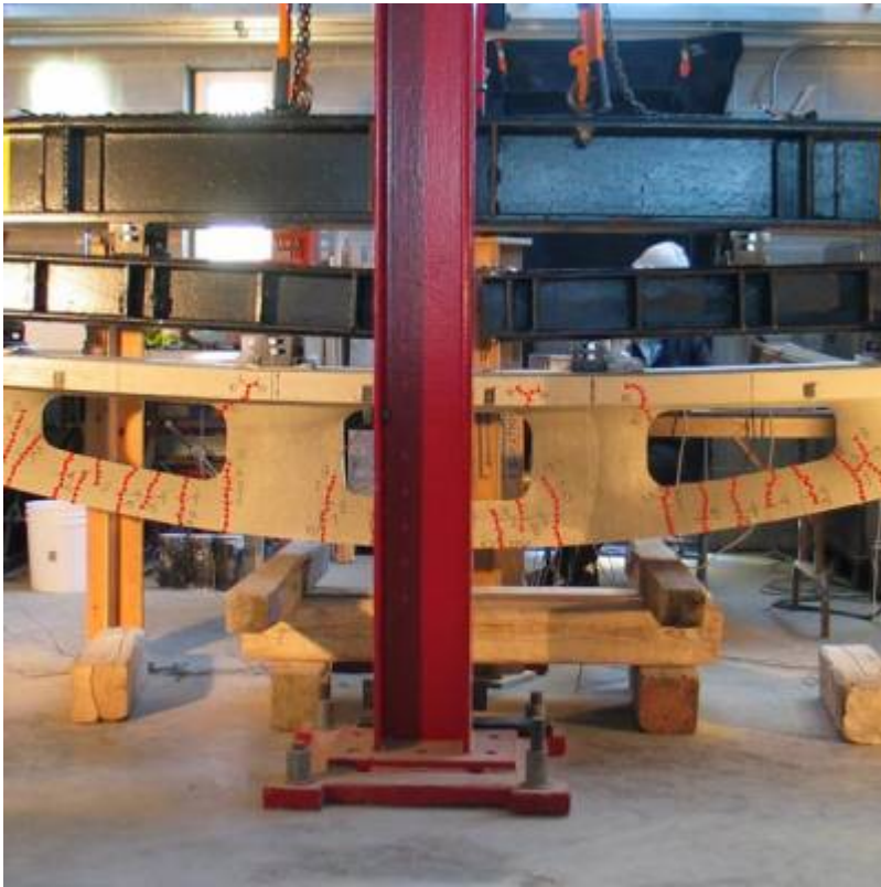
Fig. 15. Testing of variable section concrete truss.
