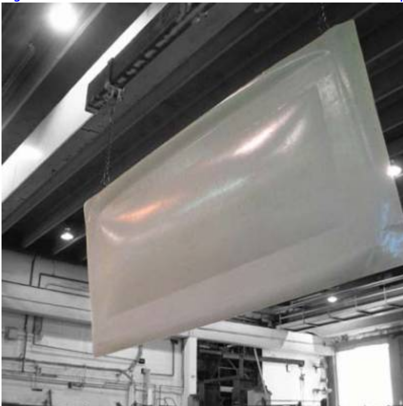
Fig. 29. Completed prototype plastic-coated mold.
