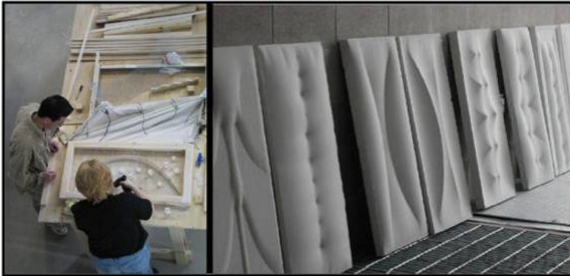
Fig. 1. Model formwork and completed plaster cast.
