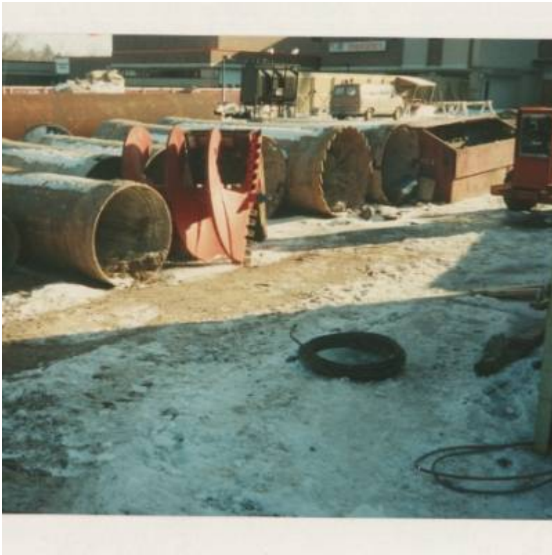
Fig. 14. Drill bits and shafts used to install drilled piers.
