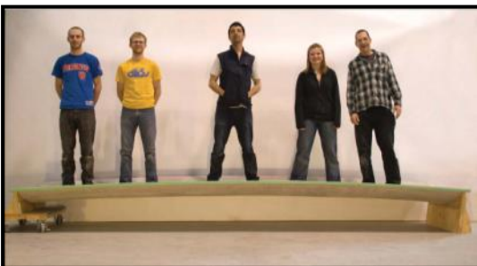
Fig. 25. Completed double-curvature funicular thin-shell vault (C.A.S.T. photo).
