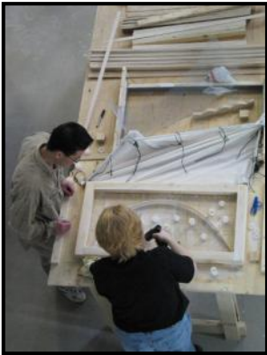
Fig. 6. Model wall panel formwork (C.A.S.T. photo).
