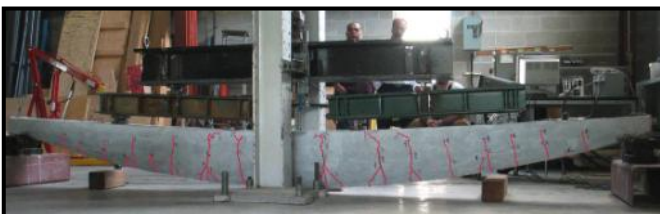
Fig. 15. Testing of variable section concrete beam (C.A.S.T. photo).
