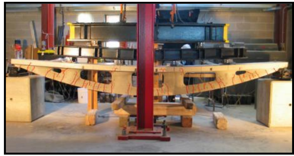
Fig. 16. Testing of variable section concrete truss (C.A.S.T. photo).
