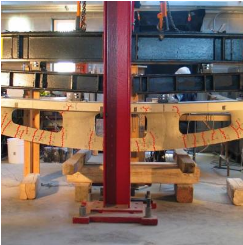
Fig. 15. Testing of variable section concrete truss.
