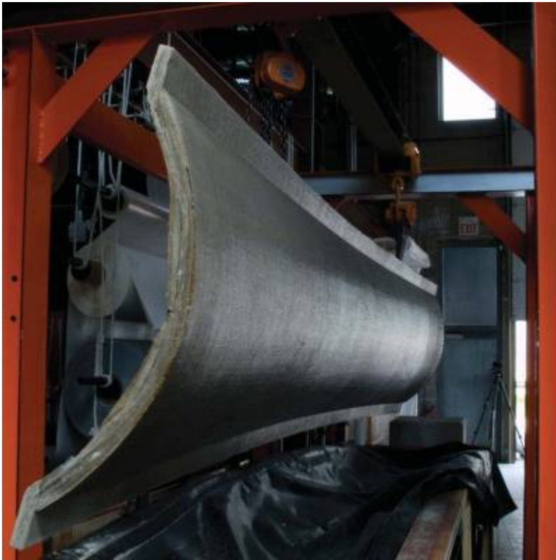
Fig. 35. Removing 3 cm (1.2 in) vault from formwork.
