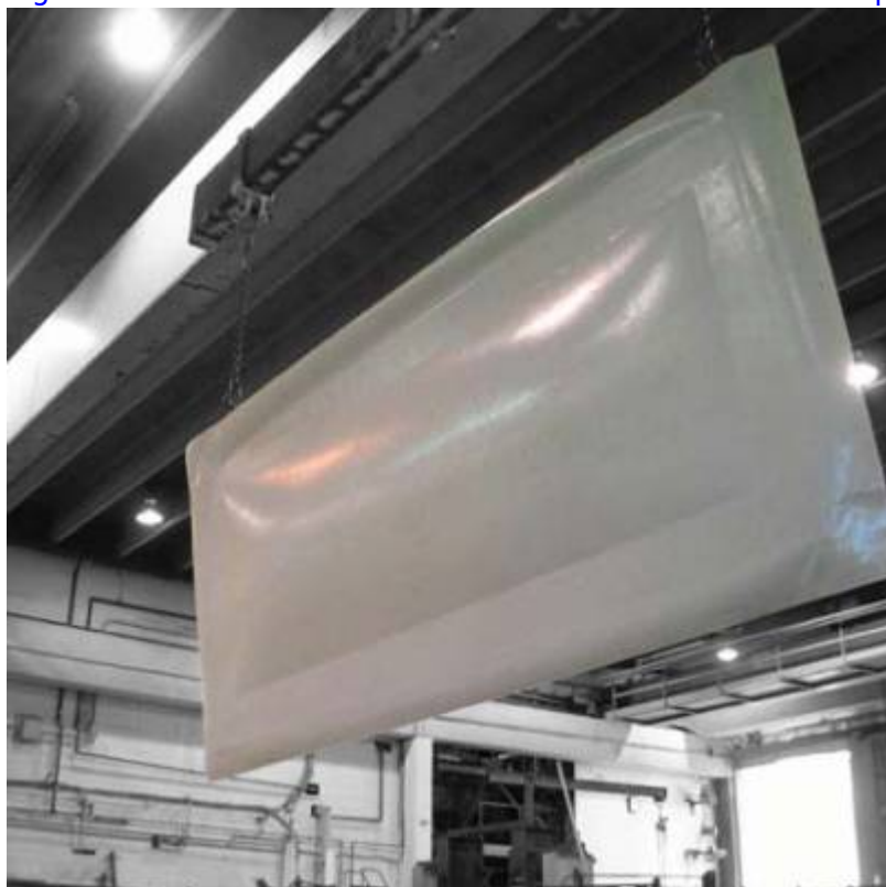
Fig. 29. Completed prototype plastic-coated mold.
