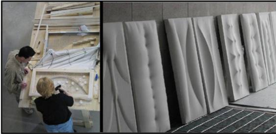
Fig. 1. Model formwork and completed plaster cast.
